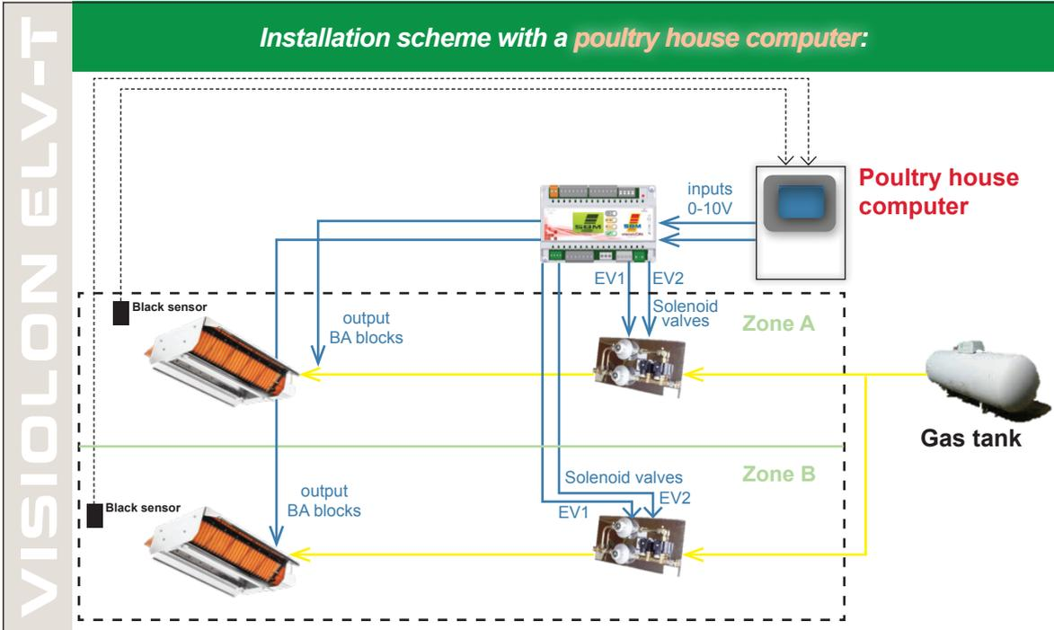
**The new added features to the control module:**
